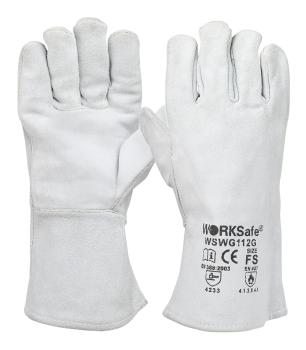
Specially designed for welders to provide high heat resistance and lasting wear. 13" length, fully lined with a one-piece leather back for optimum insulation comfort. Straight thumbs for greater flexibility.
